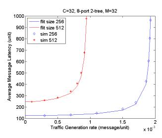
Figure 8. MCMCA for 32-cluster system with M=32 with number of cores = 1
