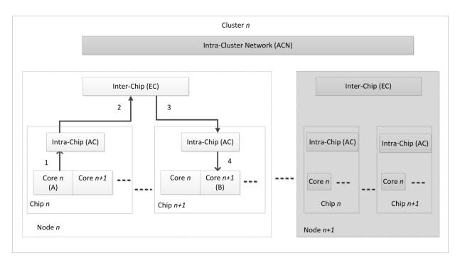
Figure 4. Message passing across processors in different chips, but within a node
