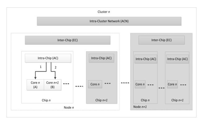
Figure 3. Communication for message passing between two processor cores on the same chip
