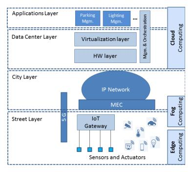
Figure 1: Layered IoT architecture
