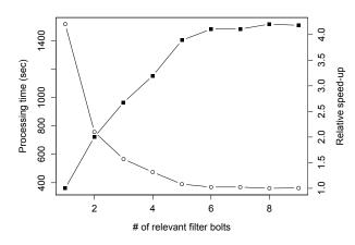
Figure 5: Processing time and relative speed-up with an increasing number of relevant filter bolts.
