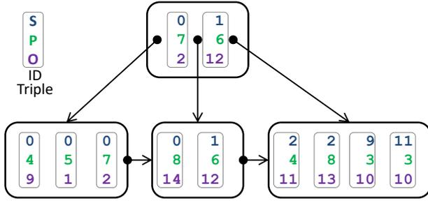
Figure 2: B<sup>+</sup>-tree containing ID triples of Listing 2 according to the SPO collation order
