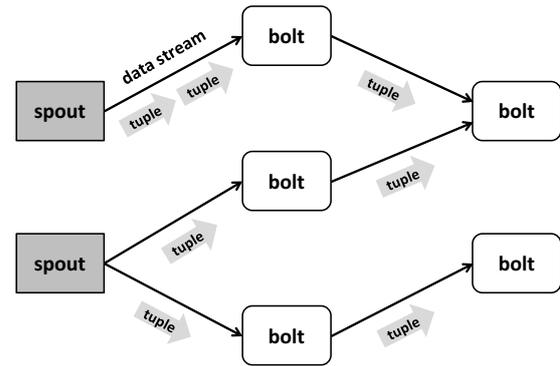
Figure 1: An illustration of Storm topology.
