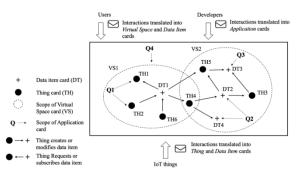
Figure 4: Logical connections between different cards
