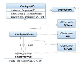
Figure 1: Business delegate (EmployeeBD and EmployeeBDImp), transfer (EmployeeTO) and JAX-WS classes in the WSC for the SOAP invocation of the WSP for employee creation. EmployeeWSB is the interface for the JAX-WS proxy for remote access to the web service broker deployed in the WSP
