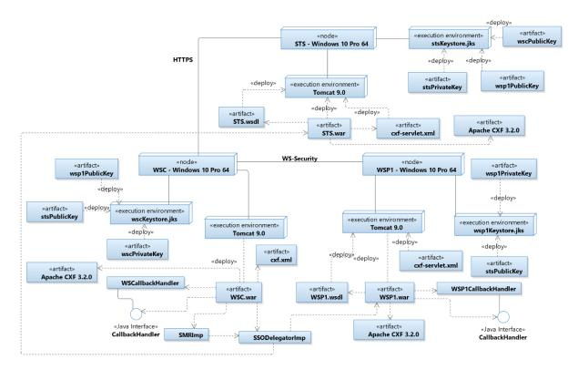
Figure 22: Deployment for SMR. For the sake of conciseness, only one platform for password change is depicted
