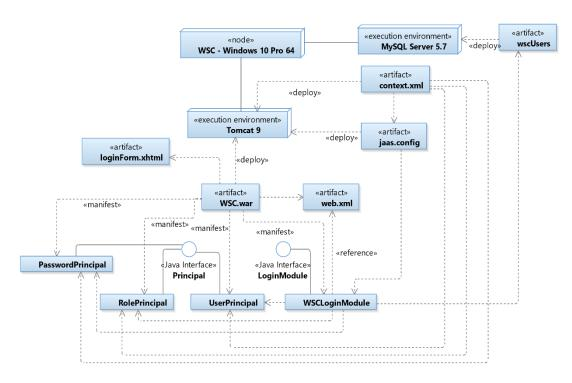
Figure 9: JAAS deployment in the WSC
