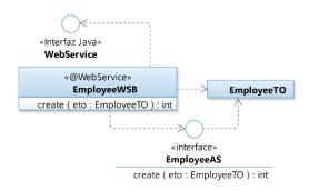
Figure 6: Web service broker (EmployeeWSB), application service interface (EmployeeAS), transfer (EmployeeTO) and JAX-WS classes in the WSP for the SOAP implementation of the web service for employee creation
