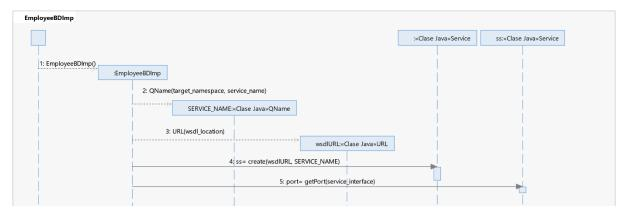
Figure 3: Configuration in the JAX-WS WSC business delegate for accessing the SOAP WSP. In this example. target\_namespace= http://wsb.employee.business, service\_name= EmployeeWSBService, wsdl\_location= http://solaris.fdi.ucm.es:8080/csp/wsdl/employeewsb.wsdl, and service\_interface= business.employee.imp.EmployeeWSB.class
