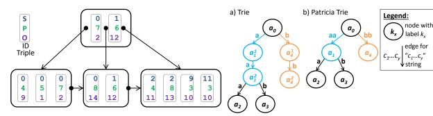
Figure 2: B<sup>+</sup>-tree containing ID triples of Listing 2 according to the SPO collation order
