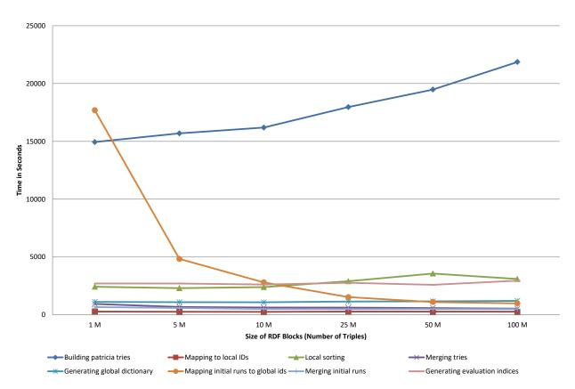
Figure 6: The processing times of the different phases of index construction for different sizes of RDF blocks
