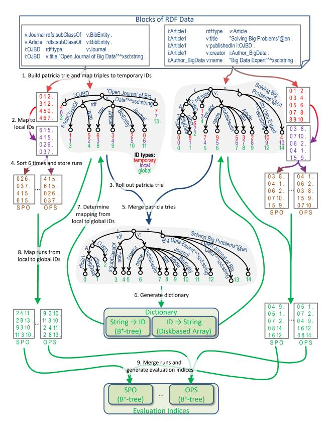
Figure 4: Overview of index construction process with example
