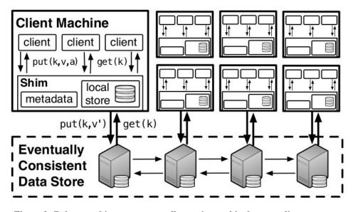
Figure 2: Bolt-on architecture: a causally consistent shim layer mediates access to an underlying eventually consistent data store [14]
