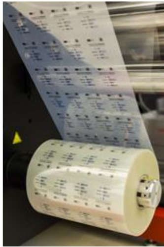
Figure 5: Roll-to-roll manufacture of an integrated printed biosensor (Used with permission from [1])
