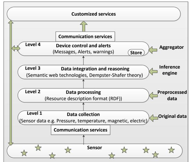
Figure 2: Multi-Level Smart City Architecture
