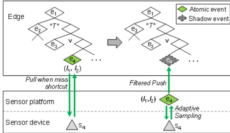
**Figure 6: Before/after atomic event  $e_4$  flows to the Beneath Layer**
