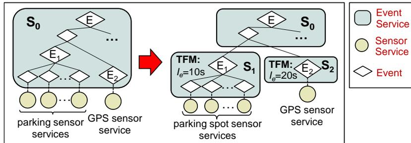
**Figure 3: TFM applied to E1 and E2 in the smart parking application**
