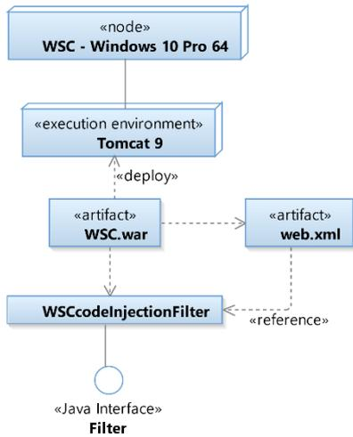
**Figure 16: Deployment for intercepting validators in the WSC**
