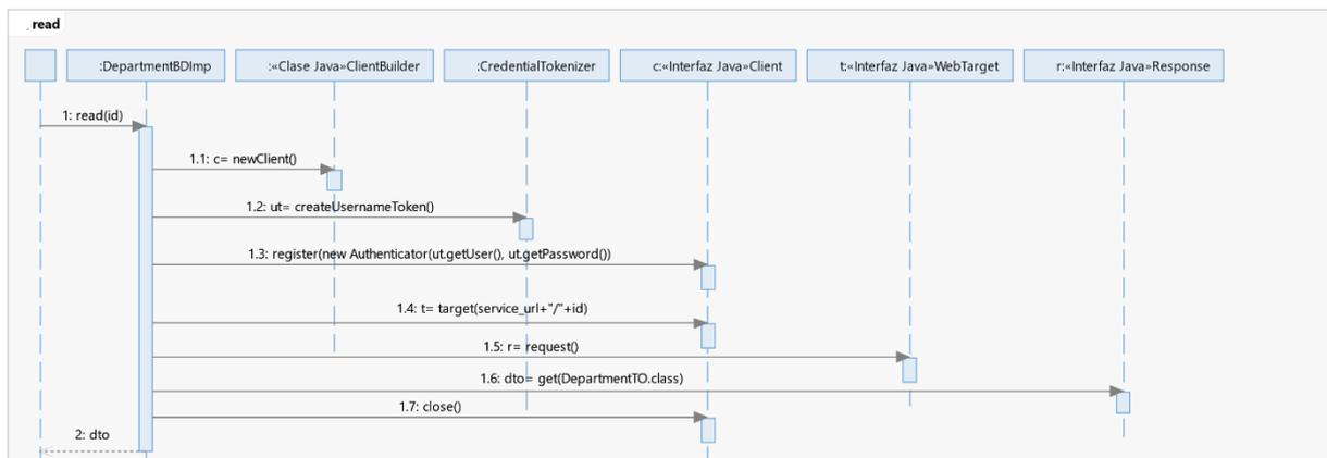
**Figure 13: Access to the REST WSP in the JAX-RS business delegate using username and password obtained from a credential tokenizer. In this example, the value of service\_url coincides with that of Fig. 5**
