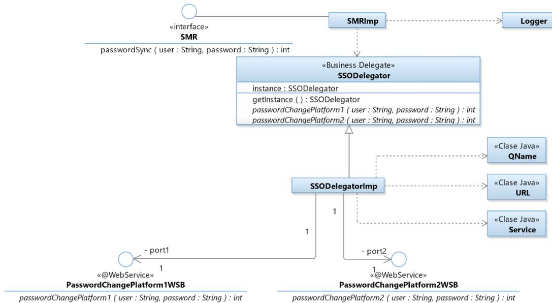
**Figure 20: The SMR (SMR and SMRImp) uses a SSO delegator (SSODelegator and SSODelegatorImp) for password synchronization. The SSO delegator has two JAX-WS interfaces (PasswordChangePlatform1WSB and PasswordChangePlatform2WSB) whose implementations give remote access to the WSPs. A Logger is used for manual transaction compensation**
