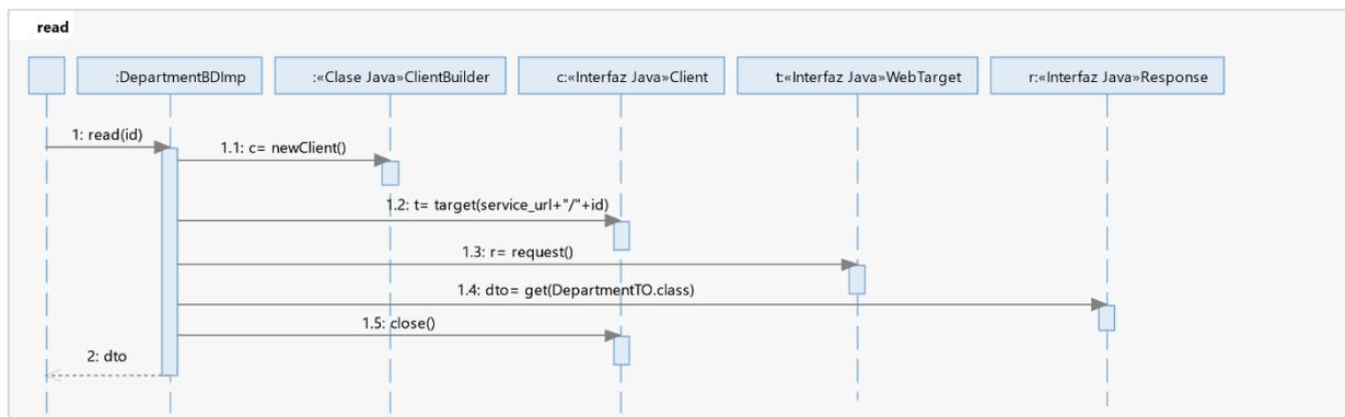
**Figure 5: Access to the REST WSP in the JAX-RS business delegate using the JAX-RS classes for remote REST access. In this example, `service_url = http://solaris.fdi.ucm.es:8080/csp/services/department/wsb`**
