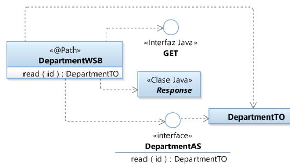
**Figure 7: Web service broker (`DepartmentWSB`), application service (`DepartmentAS`), transfer (`DepartmentTO`) and JAX-RS classes in the WSP for the REST implementation of the web service for reading a department**
