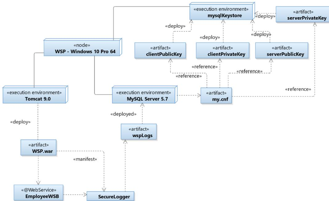
**Figure 18: Deployment for secure logger in the context of a secure service proxy. In this case, the WSP plays the role of client and MySQL Server plays the role of server. This is important in order to understand the keys deployed in the keystore used by MySQL Server (*mysqlKeystore*)**
