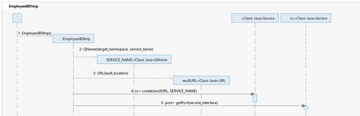
**Figure 3: Configuration in the JAX-WS WSC business delegate for accessing the SOAP WSP. In this example, `target_namespace= http://wsb.employee.business`, `service_name= EmployeeWSBService`, `wsdl_location= http://solaris.fdi.ucm.es:8080/csp/wsdl/employeewsb.wsdl`, and `service_interface= business.employee.imp.EmployeeWSB.class`**
