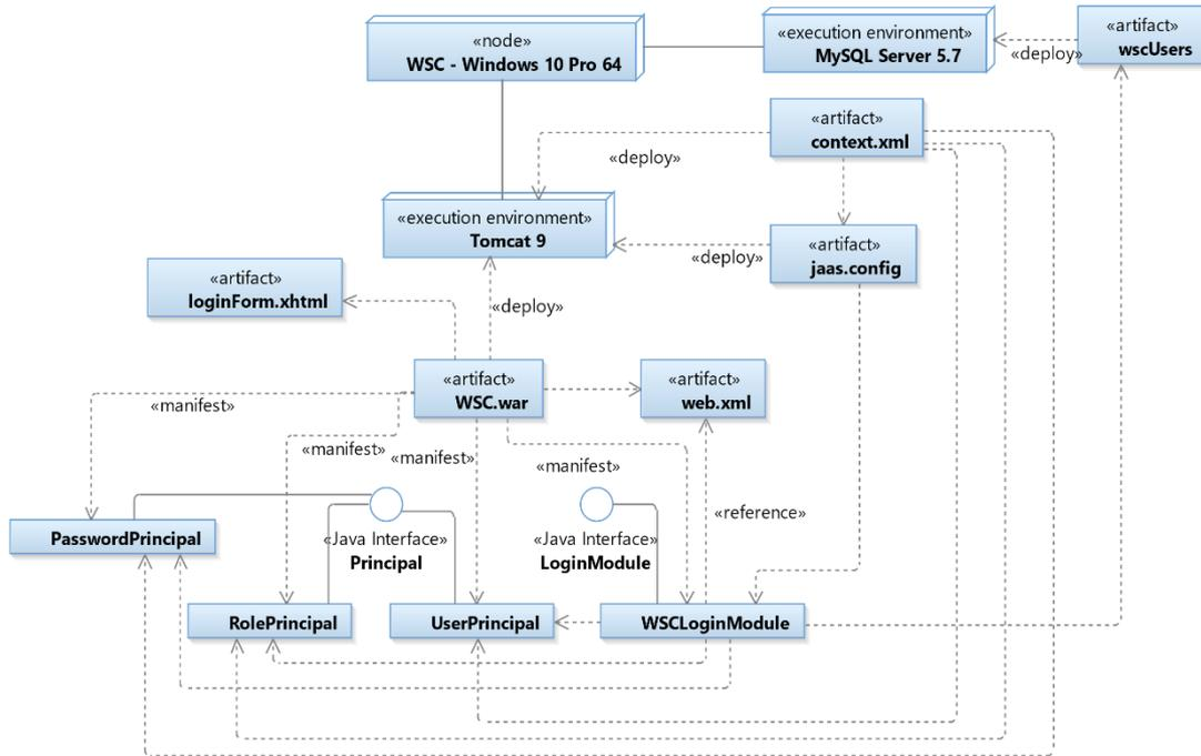
**Figure 9: JAAS deployment in the WSC**
