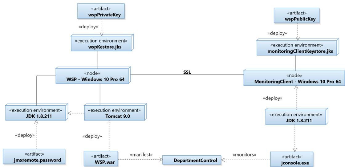
Figure 19: Deployment for dynamic server management of the WSP. In the figure, the class `DepartmentControl` is the control object used for taking account of the creation and deletion of departments
